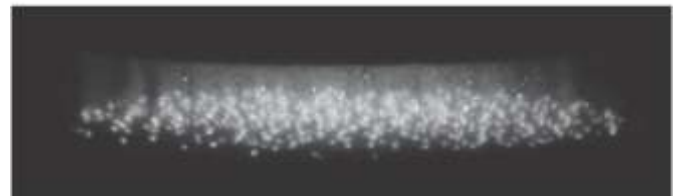
Fig.4.4. Finely dispersed vacuum arc resulting from stabilizing effect of axial magnetic field
